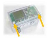
Place the unit on a flat surface and loosen the 2 nylon screws in the bottom corners to open.
